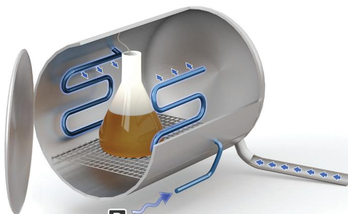
Compressed Air Inlet Chamber is Pressurized
